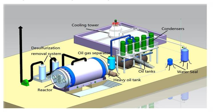
The pyrolysis plant comes in different handling capacities, depending on the mine size and the volume of waste generated. It can handle between **8 tons to 20 tons** of waste tires per day. This flexibility ensures that the plant can be tailored to meet the specific needs and waste management requirements of different mining operations.
